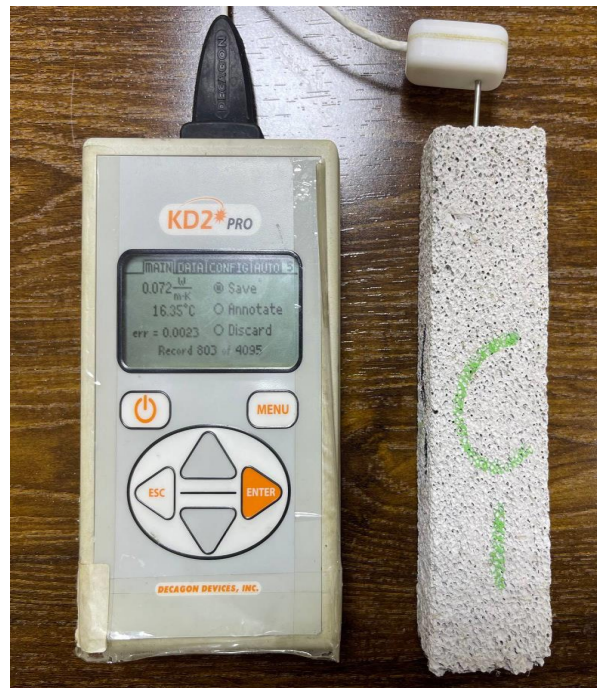
Fig. (10). The sample of AAC and the KD2 PRO device.
