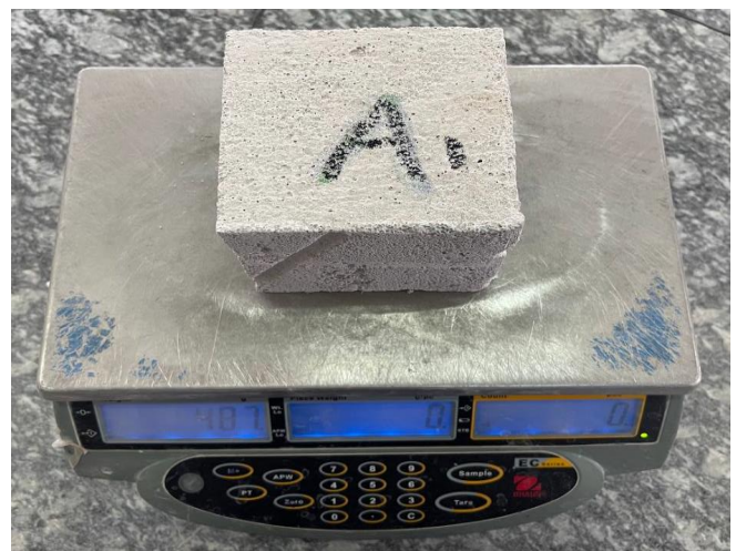
Fig. (8). The sample of AAC in the density test.
