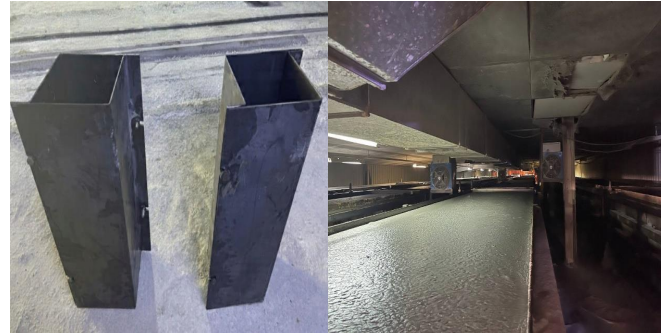
Fig. (2). The mold of AAC and the drying room.
